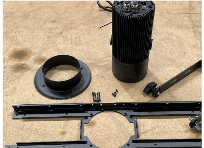
With a deep 7mm socket remove and discard the 4 nyloc nuts
