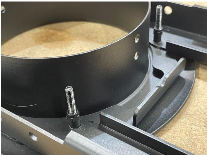
Unscrew the 4 screws completely so the fascia panel is now apart from the retaining section
